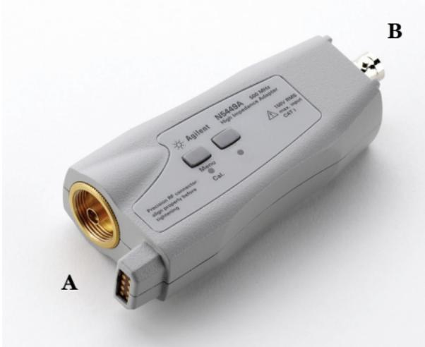
Connect one side of the adapter (**A**) to one of the input clutches on a 90000-X Series oscilloscope and connect the other side of the adapter (**B**) to the probe.
